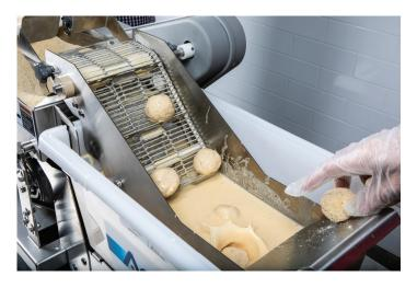
batter tank for fast, efficient coating. There's no need to drop in each food product individually. This saves on prep time and improves kitchen workplace efficiencies.
