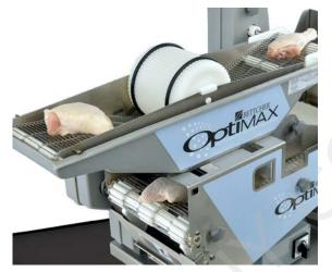
**Step 3:** The product will be coated with breading as it goes through the throat guides and under the paddle assembly. The product will exit at the front end of the breader.
