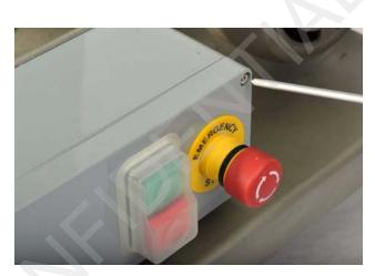
Step 9: Reinstall the drive guard covers, knobs, and locking latch.
