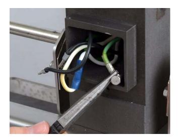
**Step 5:** <u>FOR 115V ONLY</u>: The power cord neutral (white) wire is spliced to the motor cord wire (white). Remove the splice by cutting the white wires on either side of the splice. Strip the end of the motor cord's white wire.
