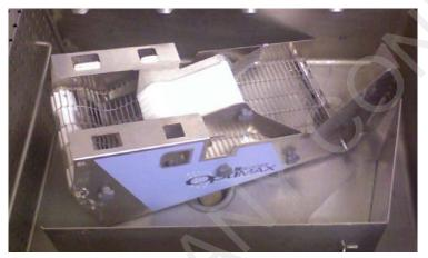
Step 10: Machine or hand wash discharge tray and pan bracket.
