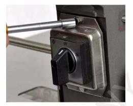
**Step 4:** Remove the power switch assembly from the switch body by releasing the red lever.
