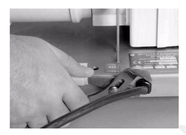
Step 17: Reinstall the drive guard covers, knobs, and locking latch.
