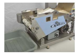
Step 3: Disengage locking latch.
