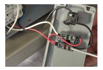
**Step 8:** Install the two screws attaching the power switch assembly to the frame.
