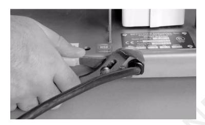
Step 17: Reinstall the drive guard covers, knobs and locking latches.
