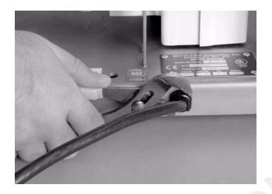
Step 15: Reinstall the drive guard covers, knobs, and locking latch.
