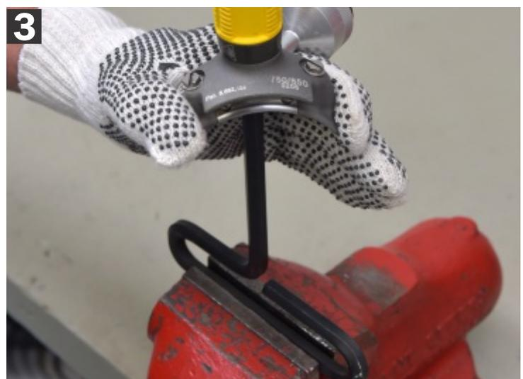
Secure the Hex Wrench in a vice and turn the trimmer to the recommended 115 - 140 lb-in of torque.
