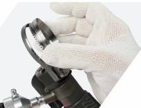
2. Make a quarterturn to close, re-tighten the screws, and you're done. Simple as that!
