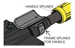
**NOTE:** The handle can be adjusted to suit the operator and the work station by pulling the handle back away from the frame and re-locating it on another set of notches on the frame tube.
