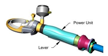
• Release the lever to turn the trimmer off.
