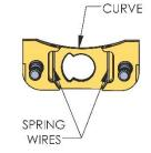
• With small tabs facing upward, insert the cam into the cam plate assembly, positioning the cam slot as shown. Note: The location of the chamfer on the cam is at the top left.
