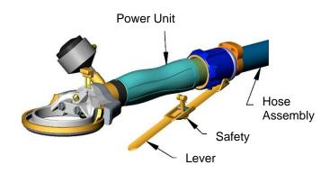
• Hold the lever against the power unit to keep the trimmer running.
