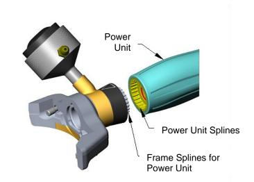
**NOTE:** The handle can be adjusted to suit the operator and the work station by pulling the power unit back away from the frame and re-locating it on another set of notches on the frame.
