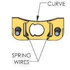
With small tabs facing upward, insert the cam into the cam plate assembly, positioning the cam slot as shown.
