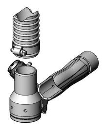
• Tighten the hose clamp screw.
