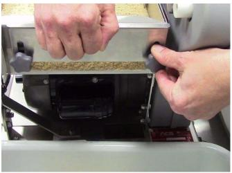
**Step 3:** Empty breading into discharge pan.
