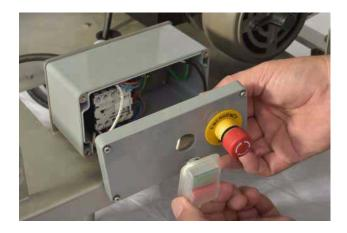
**Step 6:** Install the new switch body onto the switch and tighten the switch body screw securely.
