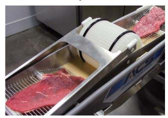
**Step 3:** The product will be coated with breading as it goes through the throat guides and under the paddle assembly. The product will exit at the front end of the breader.
