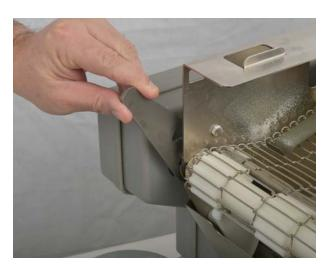
**Step 7:** Support breader at the front with left hand on the sprocket and right hand at the rear. (Place thumb through the handle with fingers supporting bottom pan.) Remove.
