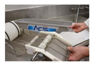
**Step 7:** After the components are dry, place the batter conveyor assembly into the batter tank.
