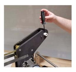
**Step 13:** Adjust the drive chain tension by allowing the weight of the motor to tension the drive chain. To avoid over tensioning the drive chain, make sure the drive chain has 3/4" slack as shown. Tighten the 4 motor mounting bolts.
