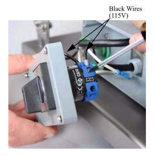
**Step 10:** Install the (4) screws attaching the power switch assembly to the frame.
