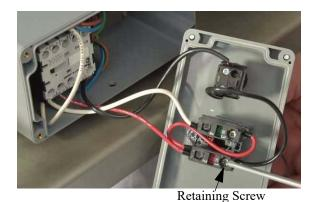
**Step 4:** Remove the power switch assembly from the switch body by loosening the switch body screw and releasing the lever.
