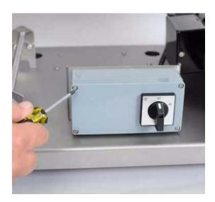
Step 11: Reinstall the drive guard covers, knobs, and locking latch.
