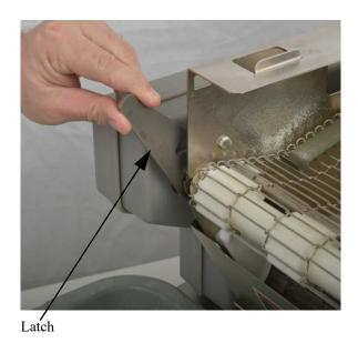
**Step 8:** Rotate spacer lock into position.
