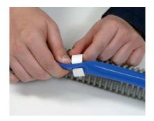
• Loosen the screw on the hose clamp.
