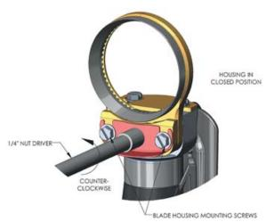
**NOTE:** There is no adjustment in the blade housing on the small tools.
