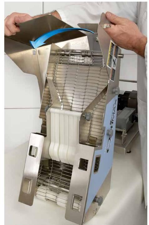
New split breeding conveyor is easier to lift — and it separates for ease of cleaning.
