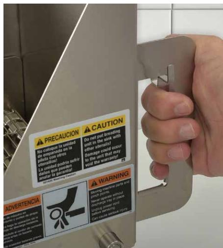
Integrated handle makes it easier to work with the breeding conveyor ... plus it's a convenient hook for holding the breeding scoop.
