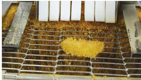
**Good Vibrations** – The ingenious vibrator springs shake off excess breading – saving on ingredient costs and extending oil life.
