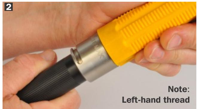
**2** Snug the retainer using the spanner wrench.
