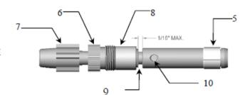
• Check the coupling cross pin (#10). If there is any free play or movement, replace the driver assembly.
