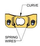
• With small tabs facing upward, insert the cam into the cam plate assembly, positioning the cam slot as shown. *Note: The location of the chamfer on the cam is at the top left.*
