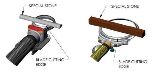
Use the Special Whizard<sup>®</sup> Steel to finish sharpening the blade. *Refer to Section 4, Steeling the Blade*.
