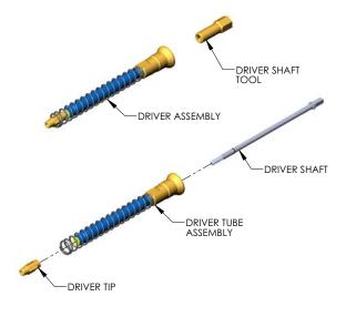
**NOTE:** Small Tool Models: X350, X360, X440, X500, X505, X500A, X564, X620, X625, X620A use a small driver tip.
