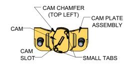
• Using a flat blade screwdriver, apply a light, downward force and turn the cam clockwise about 1/4 turn until it stops.
