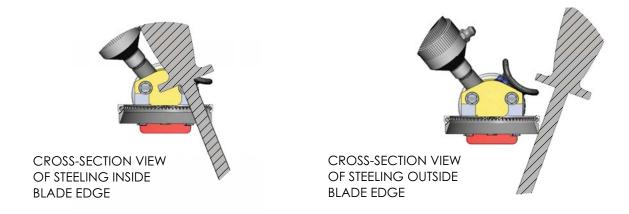
Use the steel lightly and always make the last pass of the steel on the blade on the inside surface of the blade.
