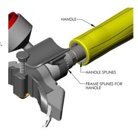
**NOTE:** The handle can be adjusted to suit the operator and the work station by pulling the handle back away from the frame and re-locating it on another set of notches on the frame tube.
