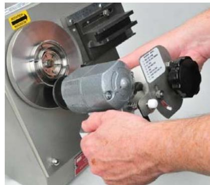
Grasp the Motor Pivot and Rotate Clockwise Against the Blade.
