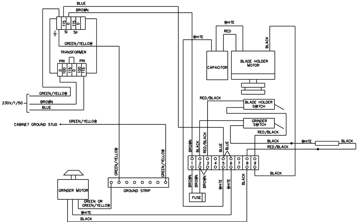
230V WIRING DIAGRAM
