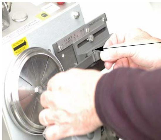
Align Front Guide Pins to Slots
