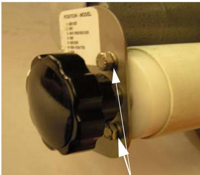
Loosen Screws to Rotate the Grinder Motor, Motor Pivot and Position Plate.
