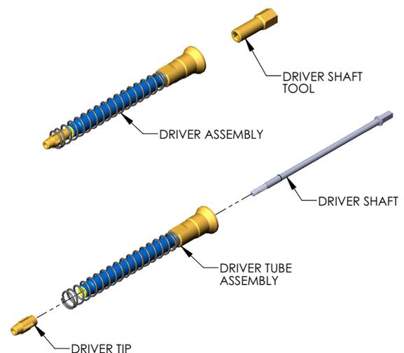
**NOTE: Large Tool Models:** X750, X850, X1000, X1300, X1400, X1500, X1850, X1880 use a large driver tip.
