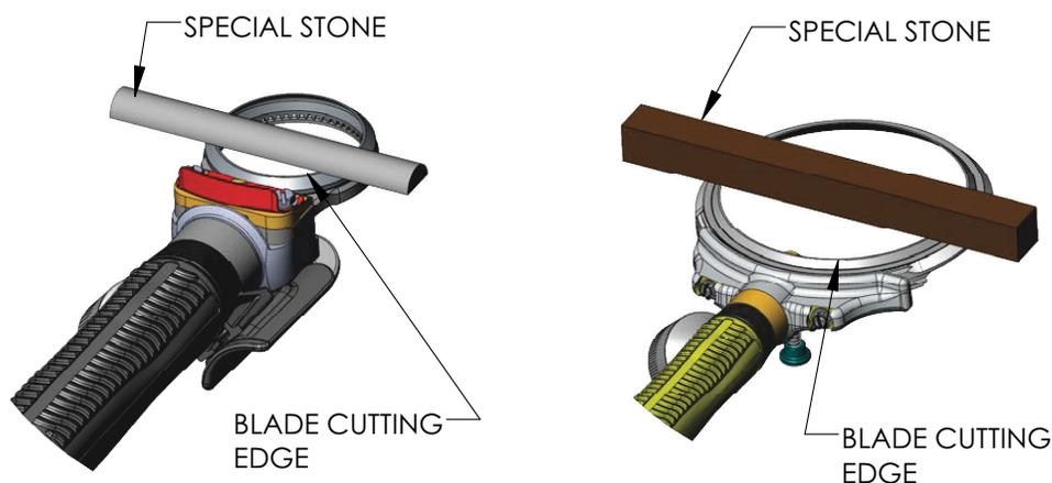
Use the Special Whizard<sup>®</sup> Steel to finish sharpening the blade. *Refer to Section 4, Steeling the Blade.*
