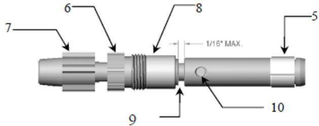
**NOTE:** The driver assembly for small diameter flexshafts have an "S" marked on the driver tip (#7).
