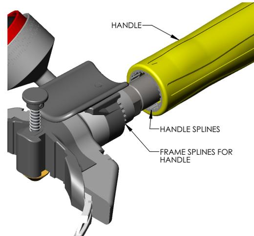
**NOTE:** *The handle can be adjusted to suit the operator and the work station by pulling the handle back away from the frame and re-locating it on another set of notches on the frame tube.*
