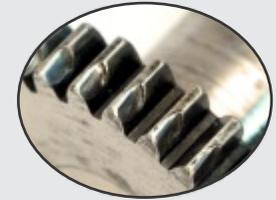
Normal wear pattern. **Replace pinion and bearing.**
