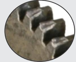
Damaged teeth caused by worn parts or improper housing adjustment.
