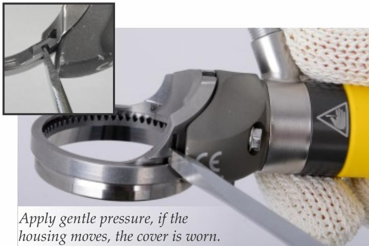
*Apply gentle pressure, if the housing moves, the cover is worn.*
