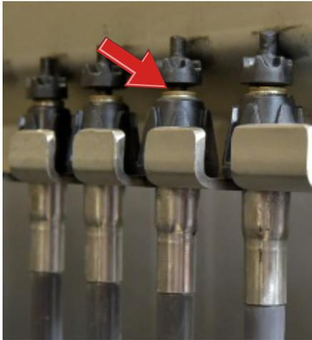
**Do NOT directly spray water in the 'gap' area of the Quantum Drivelines. Although sealed, they are not waterproof.**
