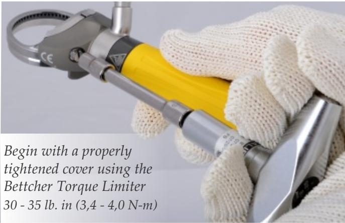
*Begin with a properly tightened cover using the Bettcher Torque Limiter 30 - 35 lb. in (3,4 - 4,0 N-m)*
