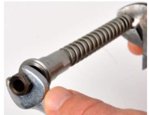
Place the Drive Shaft Tool over the square-end of the driver shaft fits into the square hole of the tool. This is a left-hand thread, so turn clockwise to loosen.
