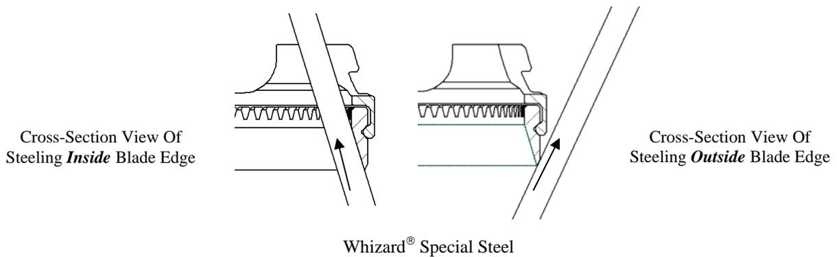
Use the steel lightly and always make the last pass of the steel on the blade on the inside surface of the blade.
